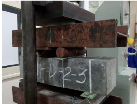
Figure 2 – Installation diagram for determining the tensile strength and crack resistance in bending
