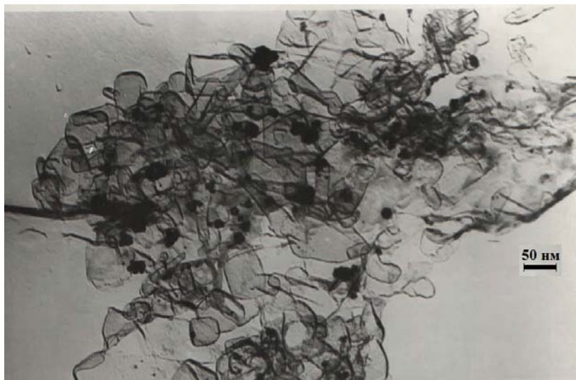
Figure 7 - Micrograph (TEM) of 1%Pd-Ag(3:1)-PAA/ZnO
