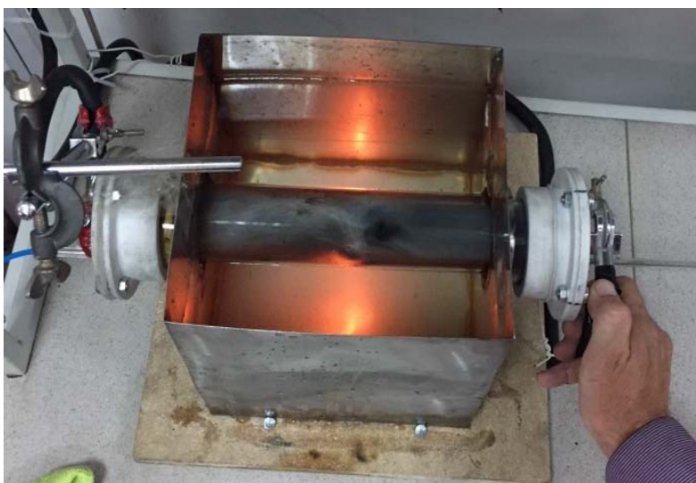
Figure 1 - Installation for producing CNTs by electrophysical method
