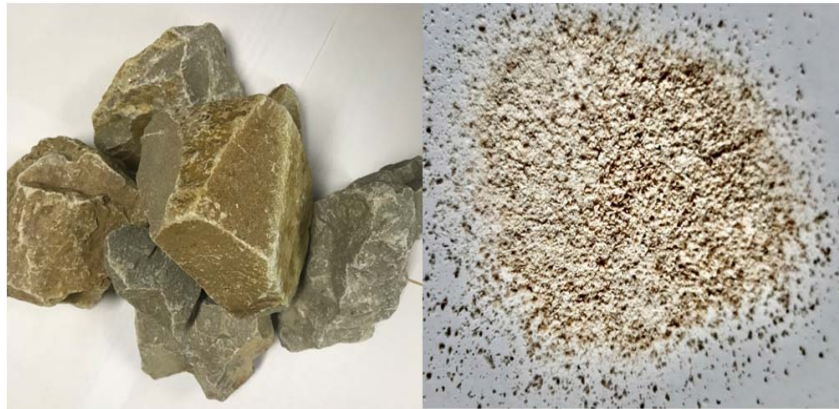
Figure 3 - A large and crushed phosphorite sample taken from the «Zhanatas» field
